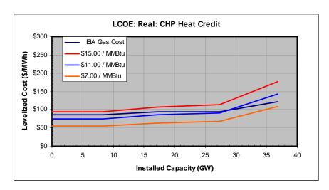
Figure 4: Real Levelized Cost of Energy (LCOE) Including a CHP Heat Credit
