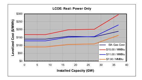
Figure 5: Real Levelized Cost of Energy (LCOE), Power Only (Not Including a CHP Heat Credit)
