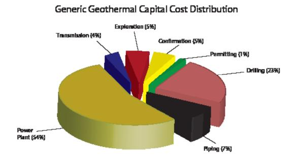
Total capital costs, including all elements of development shown in the figure above, ranged from \$3000 - \$3900 per kW for a large (100MW) plant in 2007 dollars. A smaller plant, such as the one installed at Chena Hot Springs, is expected to cost more. Considering exploration and all other elements of the Chena project, the total capital cost of the project was \$6275 per kW.
