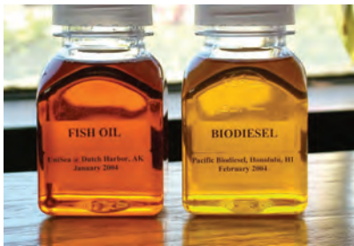
Raw fish oil and fish oil biodiesel from the Unisea plant in Dutch Harbor.
