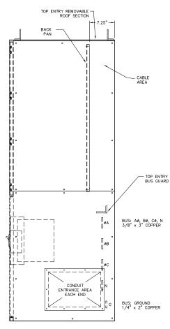
GENERATOR SWITCHGEAR - SIDE VIEW
