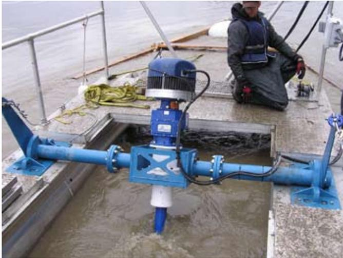
Alaska's first in-stream hydrokinetic turbine, located in Ruby.
