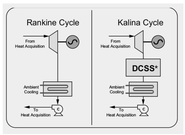
\* DCSS: Distillation – Condensation Subsystem. The DCSS consists of a series of separators, heat exchangers and pumps
