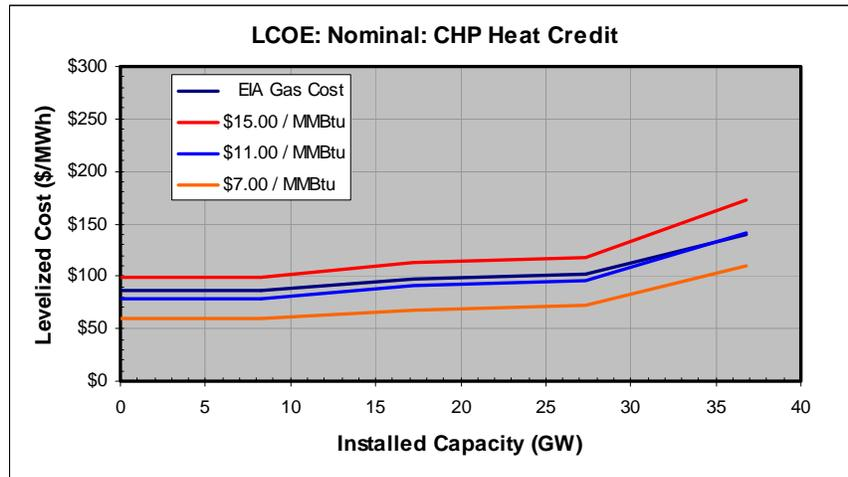
Figure 2: Nominal Levelized Cost of Energy (LCOE) Including a CHP Heat Credit
