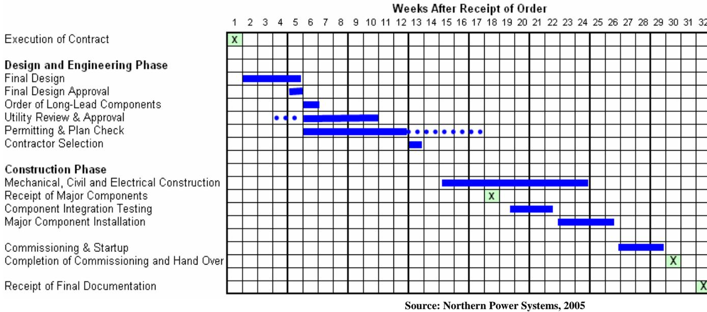
Figure 6: Estimated Timeline for Installation of a CHP System (from contract to commissioning)
